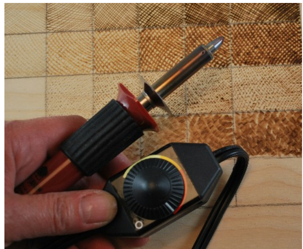
One temperature and rheostat styled burning tools are excellent beginner's units and have a nice variety of pen tip styles for any project.
